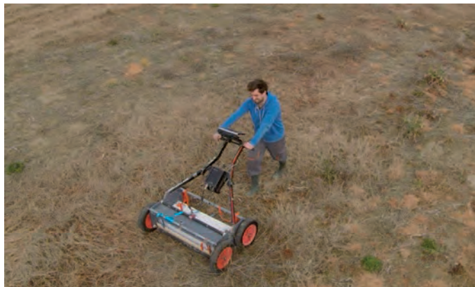
Figure 3: Le GPR en acquisition
