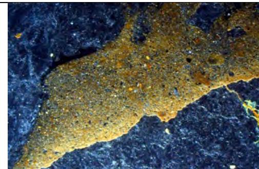
Fig. 5: As Fig 4, under OIL. Pale colour result from elutriation of iron and clay.
